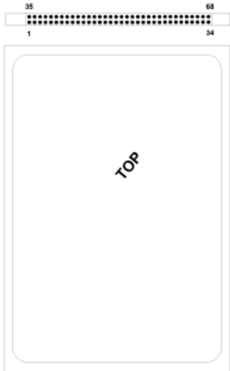
PCMCIA card showing pin assignments
