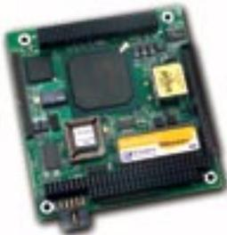
PC/104-Plus processor module with Intel 82559er 10/100 Ethernet with PXE, RPL, BOOTP, DHCP and NetWare network booting support integrated into the General Software BIOS 2000
