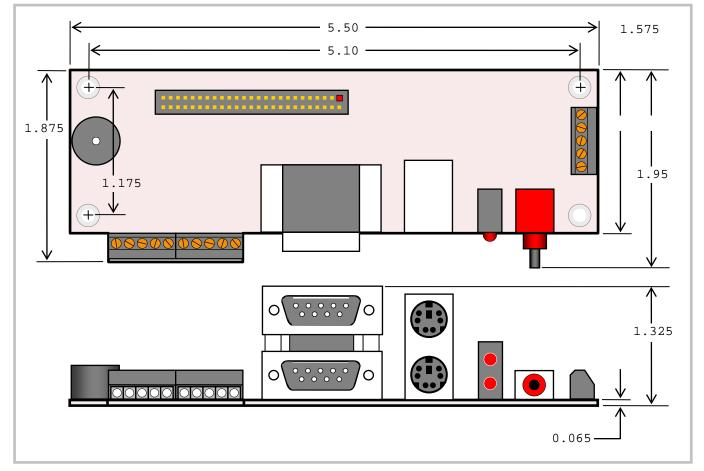
Figure 5. VL-CBR-5009 Dimensions and Mounting Holes
