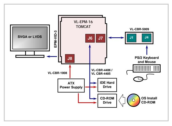
Figure 2. Typical Start-up Configuration
