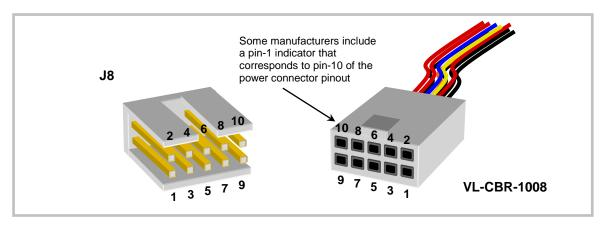
Figure 11. J8 and VL-CBR-1008 Pin Numbering
