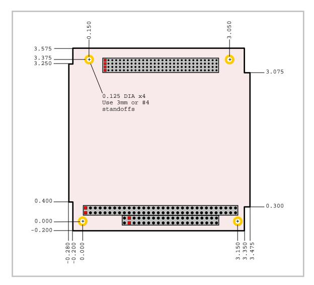
Figure 3. VL-EPM-16 Dimensions and Mounting Holes (Not to scale. All dimensions in inches.)
