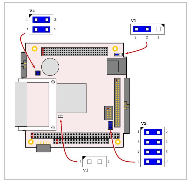
Figure 10. Jumper Block Locations
